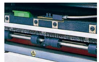
Statstrip used to dissipate static during copying
